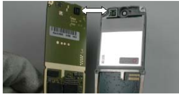
UI module and engine module after separation.
