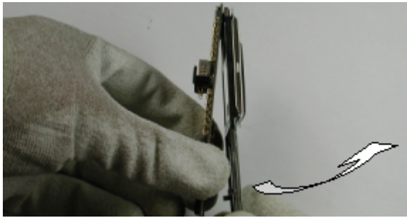
7. Remove the UI module from the engine module. Note: The UI module and the engine board are linked together by two board-to-board connectors. Be careful not to touch them.
