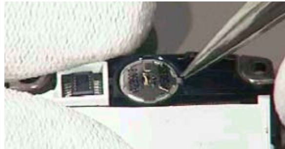
9. Remove the speaker by lifting it from the guiding pin. Note: The speaker is attached into the frame with adhesive tape. Therefore, it may not loosen easily.
