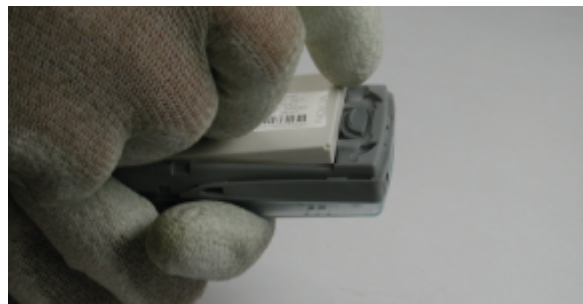
20. Pry the battery out of the phone as indicated.
